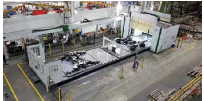
A gantry milling machine at the Bendigo facility, where it manufactures bogies for Public Transport Victoria's High-Capacity Metro Trains.
